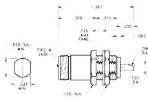
Note: Standard finish is Passivated Stainless Steel. Detail interface dimensional information can be found in the appendix.
