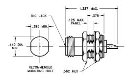
Note: Standard finish is Passivated Stainless Steel. Detail interface dimensional information can be found in the appendix.
